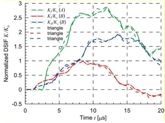
Fig.3. Normalized dynamic SIF for the branched crack with the large triangular void
