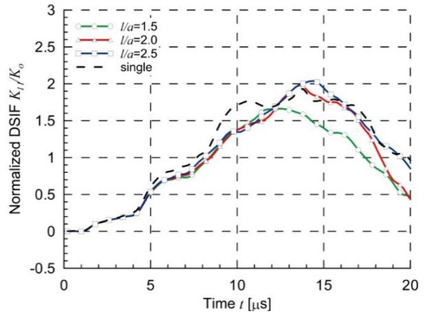
Fig. 8. Dynamic normalized SIF  $K_{II}(B)/K_o$  for the interacting inclined branches
