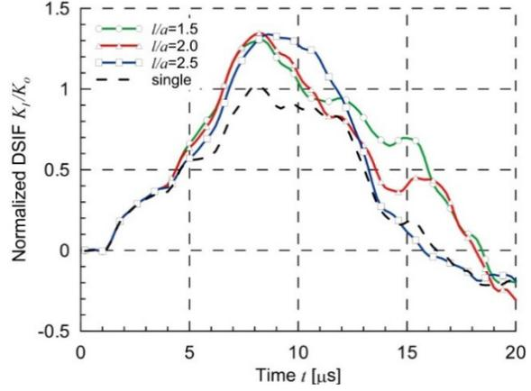
Fig. 7. Dynamic normalized SIF  $K_I(B)/K_o$  for the interacting inclined branches
