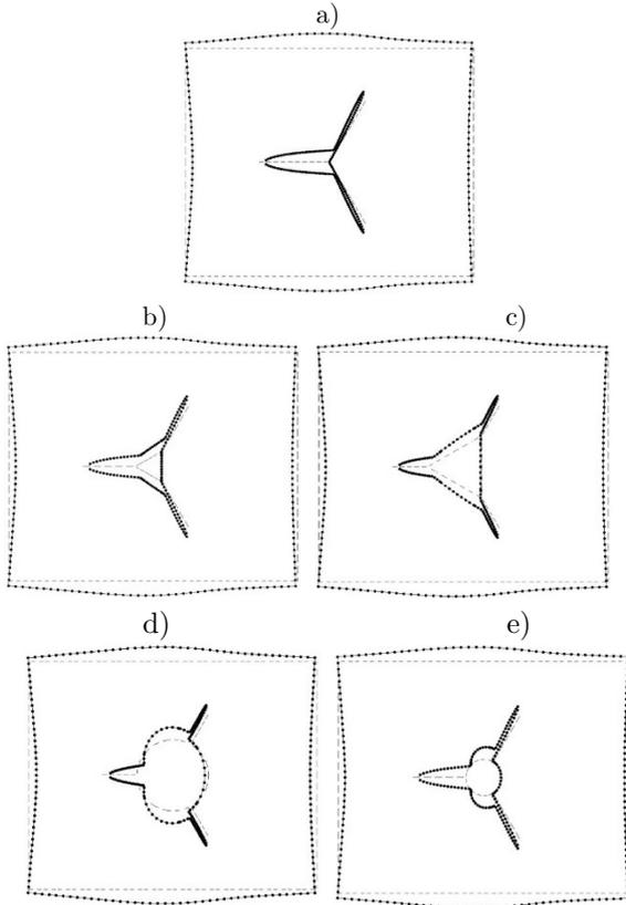
Fig. 2. Initial (dashed line) and deformed (continuous line) shape of the plate: (a) crack without the void, (b) crack with the small triangular void, (c) crack with the large triangular void, (d) crack with the small circular void, (e) crack with the large circular void
