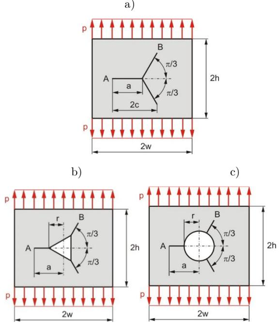
Fig.1. Single branched crack in a rectangular plate: (a) crack without a void, (b) crack with a triangular void, c) crack with a circular void in the center
