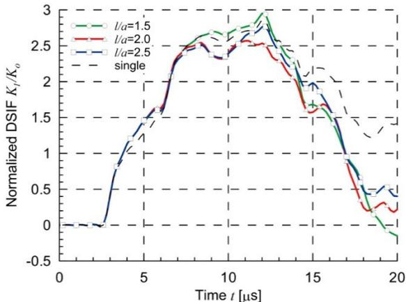
Fig. 6. Dynamic normalized SIF  $K_I(A)/K_o$  for the horizontal interacting branches
