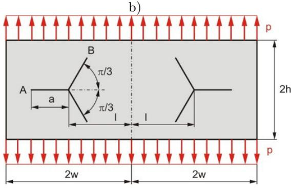
Fig. 5. Two interacting branched cracks: (a) interaction of horizontal branches, (b) interaction of inclined branches
