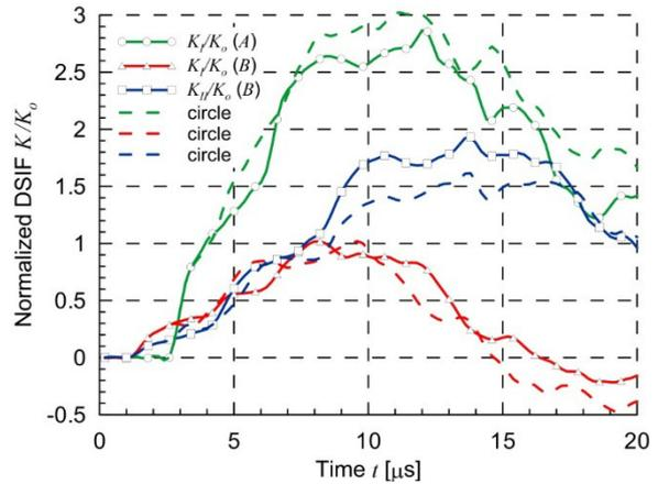
Fig. 4. Normalized dynamic SIF for the branched crack with the large circular void
