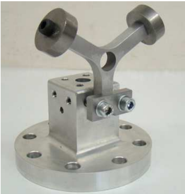
Fig. 12. Experimental specimen and holder presented by Česnik in [17]
