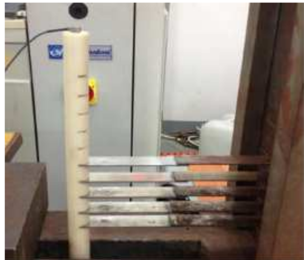
Fig. 8. View of the blade mounted on the movable head of the shaker [13]
