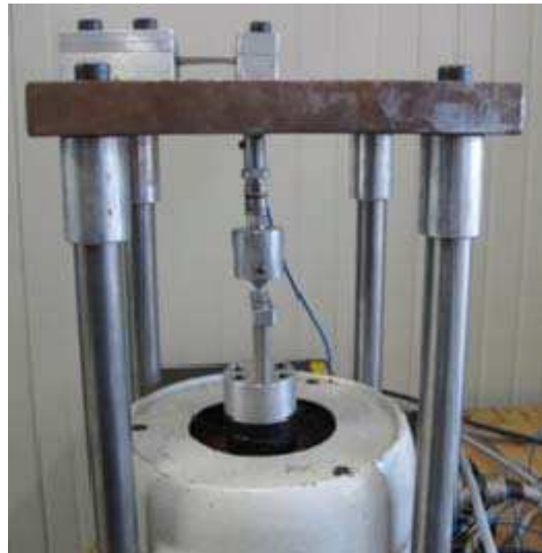
Fig. 10. Fatigue test stand developed by Ghielmetti [6]
